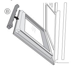
On the open side of the door strip (B) there is a guide bar (C). This must be pressed between the outer side of the door and the corner (D). The seal (E) must audibly click into place.
